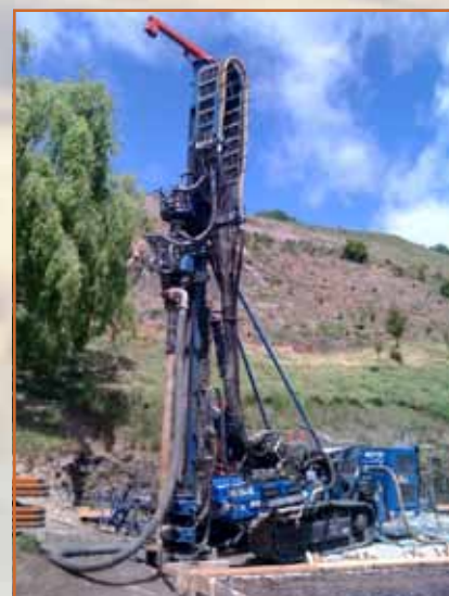
A drilling rig is needed on site to install a vertical ground source system.
